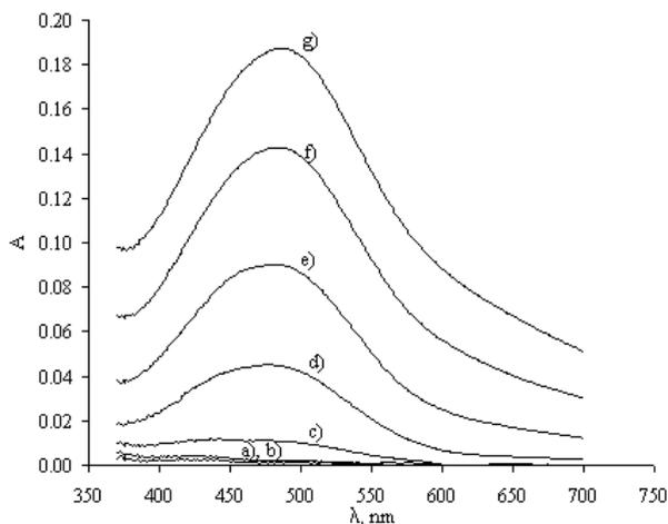
**Figure 2.** Spectra of the reaction mixture at various stages of the reaction progress: a) no enzyme added; b) after 1 min; c) after 3 min; d) after 5 min; e) after 6 min; f) after 8 min; g) after 10 min
