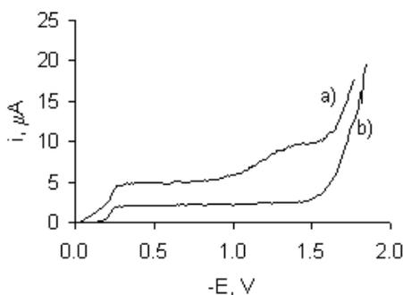
**Figure 4.** NP polarograms recorded in the studied solution 10 min after the enzymatic reaction was initialised a) before removal of oxygen; b) after removal of oxygen. Tyrosine concentration:  $C_{\text{TYR}} = 0.075 \text{ mmol L}^{-1}$
