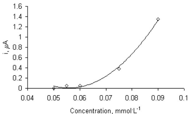
**Figure 7.** The dependence of quinone reduction NP currents on the initial substrate concentration (conditions as in Figure 5)
