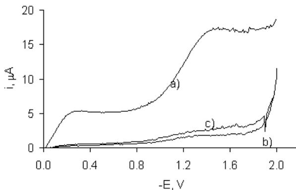
**Figure 3.** NP polarograms recorded in the studied solution before enzymatic reaction: a) 0.1 mol L<sup>-1</sup> phosphate buffer (pH = 6.8); before removal of oxygen; b) 0.1 mol L<sup>-1</sup> phosphate buffer (pH = 6.8); after removal of oxygen; c) 0.1 mol L<sup>-1</sup> phosphate buffer (pH = 6.8); after removal of oxygen; tyrosine concentration: C<sub>TYR</sub> = 0.075 mmol L<sup>-1</sup>
