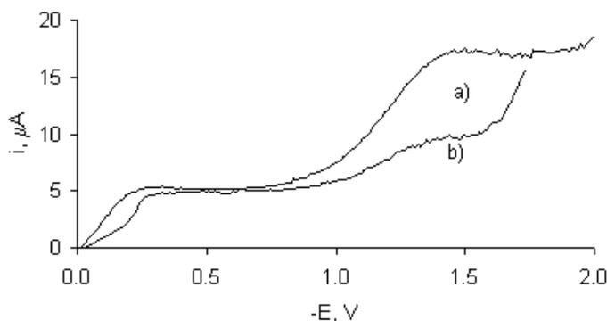
**Figure 5.** NP polarograms recorded before (a) and after (b) the enzymatic reaction, without the preliminary oxygen removal. Tyrosine concentration:  $C_{\text{TYR}} = 0.075 \text{ mmol L}^{-1}$
