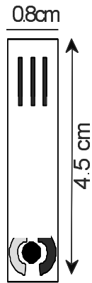
Figure 1. A scheme of a carbon screen-printed electrode
