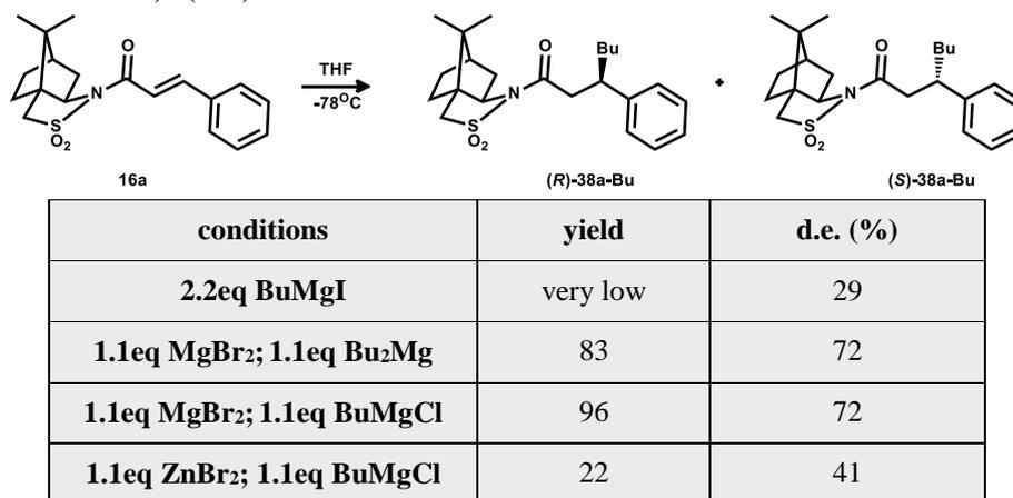
**Scheme 15.** The use of 1 equiv. of Grignard reagent in the presence of 1 equiv. of inorganic salt in 1,4-addition reaction.
