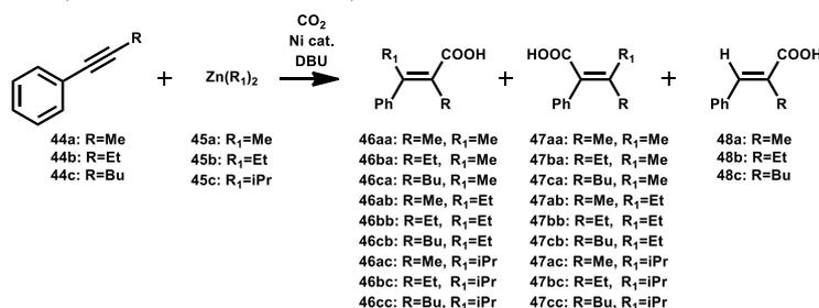
**Scheme 21.** The influence of substituents in alkyne and organozinc compounds on the carbometallation reaction.
