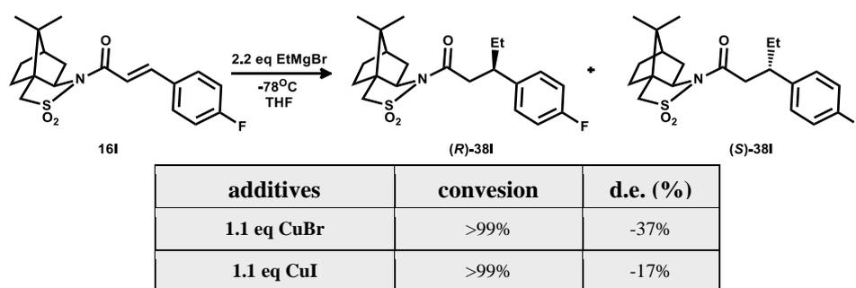
**Scheme 16.** The use of copper salts in 1,4-addition reaction of Grignard reagents.
