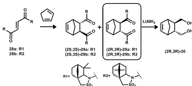
**Scheme 10.** The [4+2]cycloaddition reaction of fumaroyl derivatives of sultams **28a** and **28b**.
