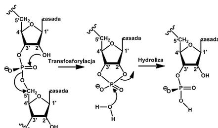
**Scheme 1.** The mechanisms for RNA cleavage.
