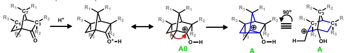
**Scheme 7.** The mechanism of sulfonation reaction (part 1).
