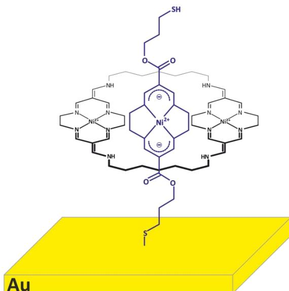
Fig. 1. Scheme of rotaxane on electrode surface [H1].
