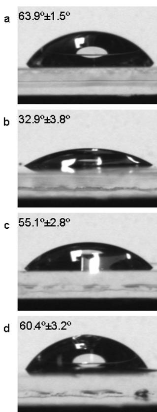
Fig.4. Images of HEPES droplet ( $20 \mu\text{l}$ ) on the surface of electrode modified with peptide (a), after phosphorylation (b), after adsorption of silver ions  $\text{Ag}^+$  (c), after reconstruction of the surface using alkaline phosphatase (d).
