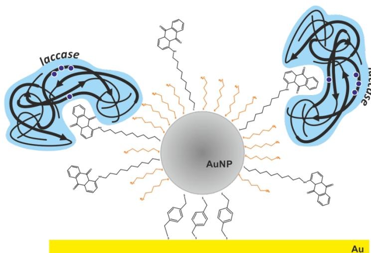
Fig.13. Scheme of the system for catalytic reduction of oxygen [H8].
