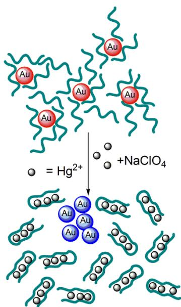
Fig 14. Scheme of mercury ions detection using AuNPs modified with DNA [H9].
