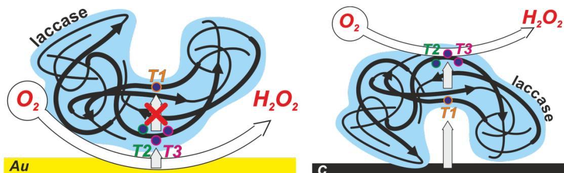
Fig 9. Scheme of laccase orientation on different type of electrodes
