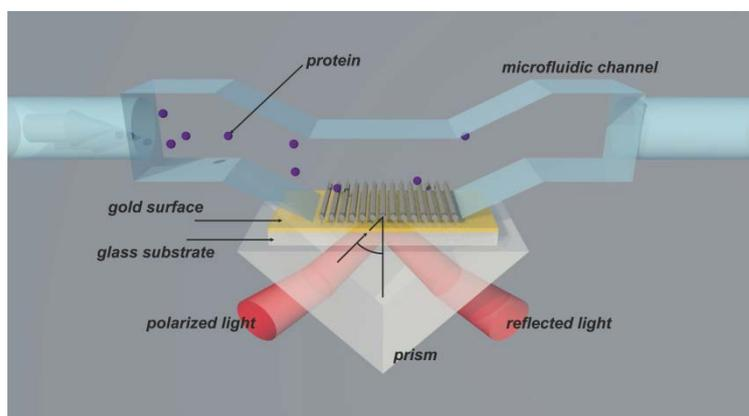
Fig. 7. Scheme of the surface plasmon resonance principles.
