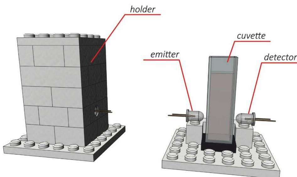
**Figure 1.** Stand made of LEGO bricks that allows permanent fixing of the light-emitting diodes in photometric measurements.
