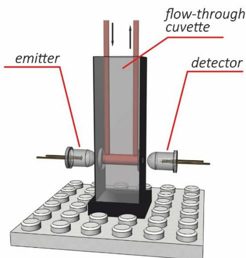
**Figure 3.** A flow-through cell used in a preliminary photometric studies with PEDD.
