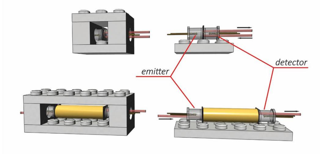
**Rysunek 7.** *Photometric flow-through cells with light-emitting diodes, made without gluing. (Left side: - assembled, Right side: disassembled)*
