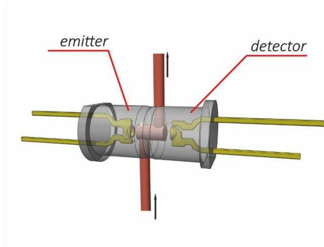
**Figure 5.** Flow-through cell made of two LEDs permanently connected to each other.
