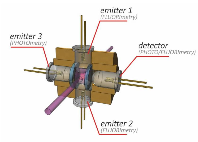
**Figure 12.** Flow-through cell allowing dual photometric/fluorimetric detection.
