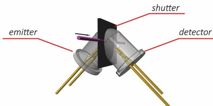
**Rysunek 6.** *Flow-through cell made of two LEDs connected permanently for the fluorimetric measurements*
