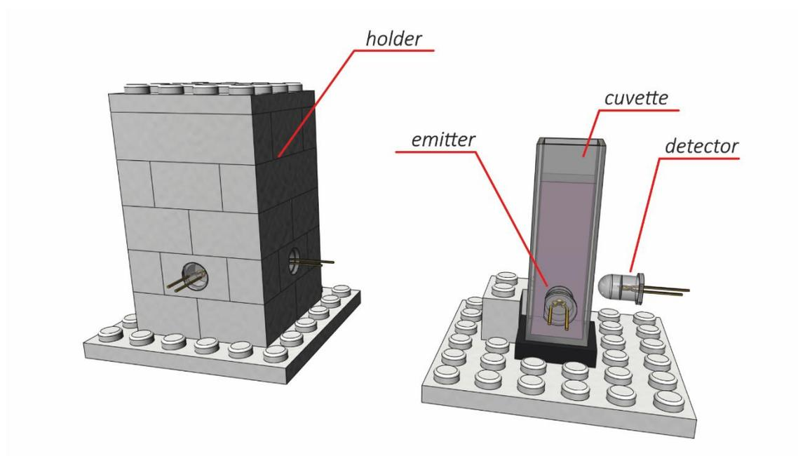
**Figure 2.** Stand made of LEGO bricks that allows permanent fixing of the light-emitting diodes in fluorimetric measurements.
