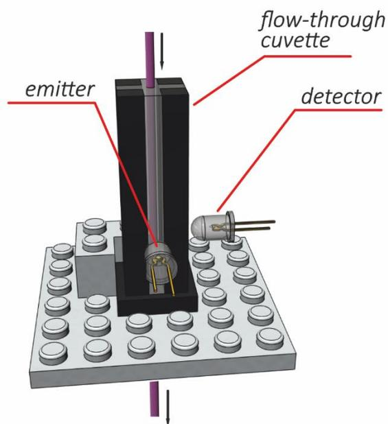
**Figure 4.** A flow-through cell used in a preliminary fluorimetric studies with PEDD.
