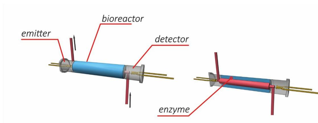
**Figure 8.** Flow-through cell with integrated enzymatic bioreactor. Left: complete cell , Right: cross-section of the cell.
