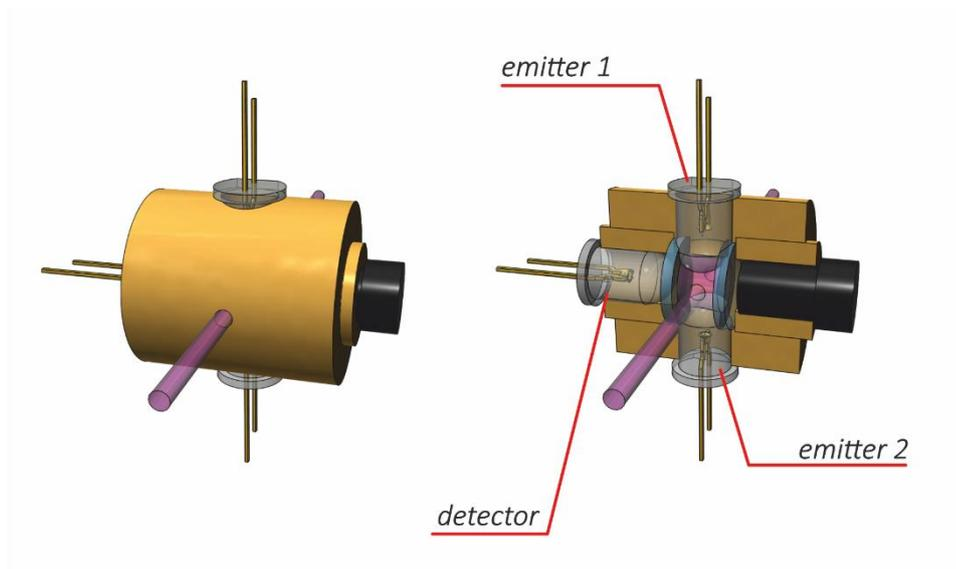
**Figure 10.** *Photometric flow-through cell (cross-section) with unmodified interchangeable LEDs, which allows placing bioreactor and/or chemosensitive layer/layers inside.*
