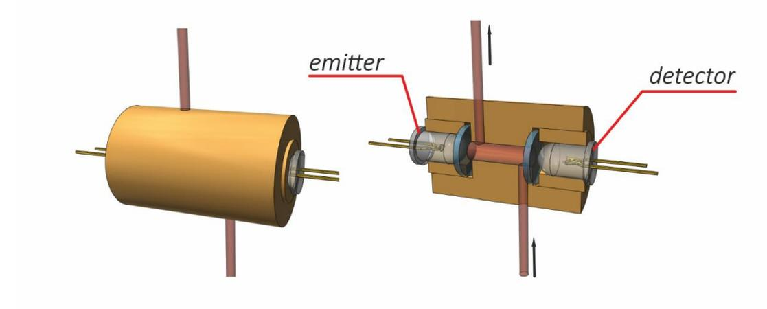
**Figure 9.** Flow-through photometric cell with unmodified interchangeable LEDs.
