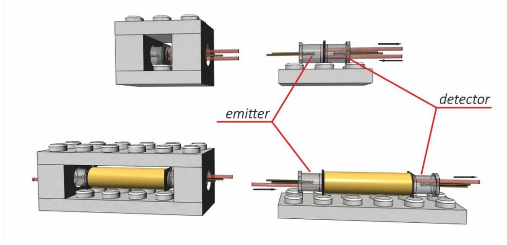
**Rysunek 7.** *Photometric flow-through cells with light-emitting diodes, made without gluing. (Left side: - assembled, Right side: disassembled)*
