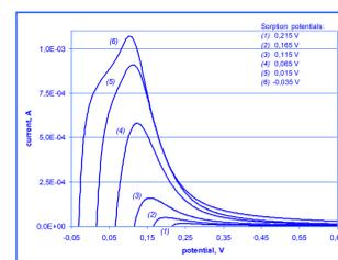
Fig. 4b. Oxidation peaks recorded after hydrogen sorption (300 s) at different potentials for 53,4% Pd-Au alloy; scan rate 0,01 V/s.
