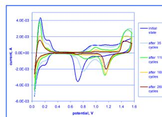
Fig. 6. Voltammograms of Pd-Au electrode (0,05 V/s) recorded after successive cycling in the potential range from 0,365 to 1,565 V at scan rate 0,1 V/s. Initial bulk palladium content 73,2 %.
