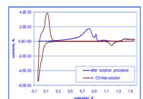
Fig. 8b. Voltammograms for Pd-Au alloy (rich in gold on the surface); scan rate 0,01 V/s. Sorption procedure: 300 s - hydrogen absorption at -0,035 V; 600 s - CO adsorption at -0,035 V; 300 s - CO removal with Ar.
