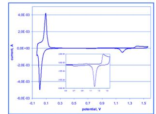
Fig. 7. Voltammogram of Pd-Au electrode (0,01 V/s), impoverished in Pd during electrochemical treatment. The region of oxygen adsorption/desorption is shown separately.
