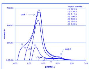
Fig. 4a. Oxidation peaks recorded after hydrogen sorption (300 s) at different potentials for 72,3% Pd-Au alloy; scan rate 0,01 V/s.
