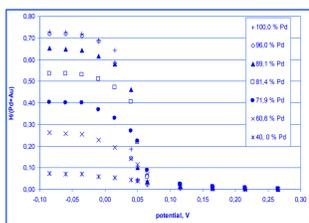
Fig. 1. Dependence of H/(Pd+Au) ratios on electrode potential for Pd-Au alloys of various bulk compositions. Time of hydrogen absorption 300 s; scan rate during hydrogen electrooxidation 0,01 V/s.
