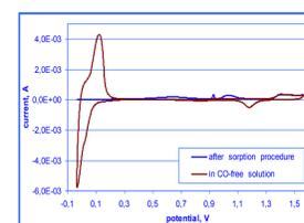
Fig. 8a. Voltammograms for Pd-Au alloy (rich in gold on the surface); scan rate 0,01 V/s. Sorption procedure: 600 s - CO adsorption at 0,415 V; 300 s - CO removal with Ar; 300 s - hydrogen absorption at -0,035 V.
