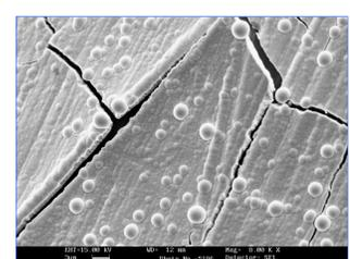
Fig. 10. SEM image of Pd-Au alloy surface taken after hydrogen absorption/desorption procedure.
