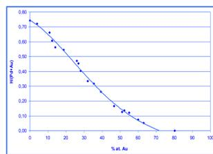
Fig. 2. Influence of bulk gold content on maximum H/(Pd+Au) ratios. Time of hydrogen absorption 300 s; scan rate during hydrogen electrooxidation 0,01 V/s.
