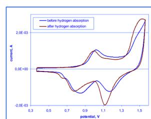
Fig. 9. Influence of hydrogen absorption/desorption experiments on the shape of voltammogram of Pd-Au alloy; scan rate 0,1 V/s.
