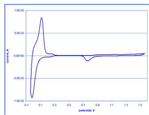
Fig. 3. Voltammogram of 74,0%Pd-Au alloy at scan rate 0,01 V/s.
