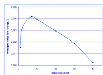
Fig. 5. Dependence of hydrogen oxidation charge on scan rate for 79,3% Pd-Au alloy. Potential of hydrogen absorption -0,035 V; absorption time 300 s. Alloy layer thickness 2,9 nm.
