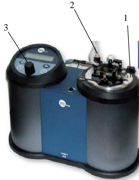
Figure 11. Setaflash Apparatus for the flash point determination in closed crucible: 1 – brass crucible placed in a steel vessel, 2-thermometer, 3-stirrer.
