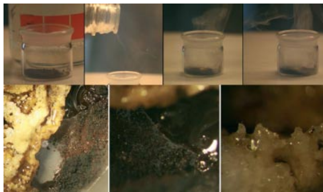
Fig. 3 The progress of reaction between AgF 2 and fuming H 2 SO 4 (top) and the products of reaction (bottom). Dense colourless H 2 SO 4 × SO 3 is added drop by drop to the reaction vessel containing brown AgF 2 .
