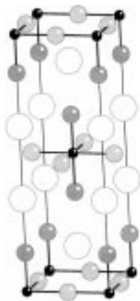
Figure 8. Unit cell of [CsF] 2 [AgF 2 ]. Note the elongated octahedral coordination of the \text{Ag}^{\text{II}} centers; Ag: black spheres, Cs: white spheres, F: gray spheres.
