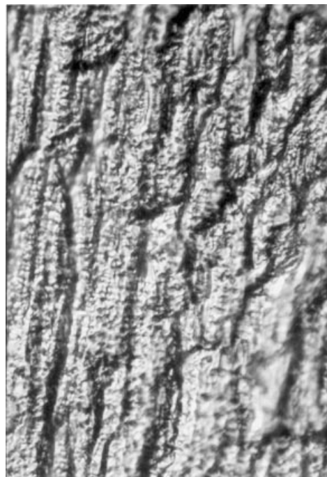
Figure 3. Typical morphology of Cu surface after the roughening according to the new OR procedure (ii), when the electrode is oscillating between both the active and the passive state. Magnification 1000\times .
