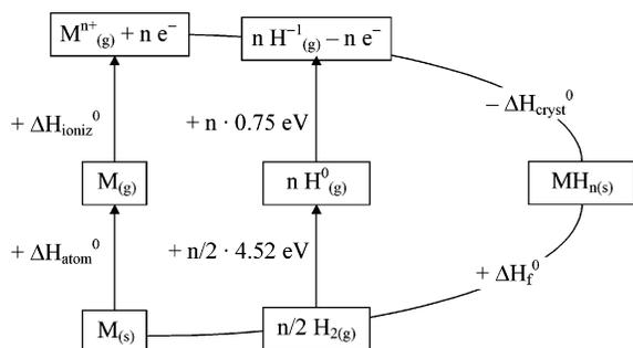
**Figure 6.** The Born–Haber cycle for the formation of  $(MH_n)_n$ .
