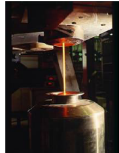
Two-step calciner / hot crucible vitrification process
