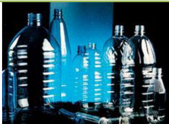
Conversion using blow molding
